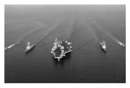
Figure 7.6 Large-scale Kelvin wakes. (Image source: US Navy).
